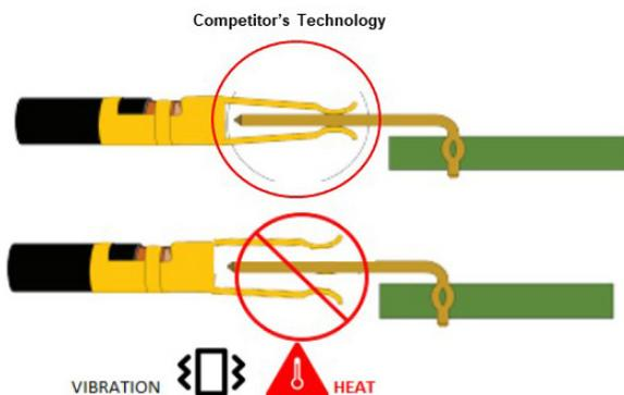
Standard Box & Blade designs only provide 2 points of contact and spring squeezes blade
