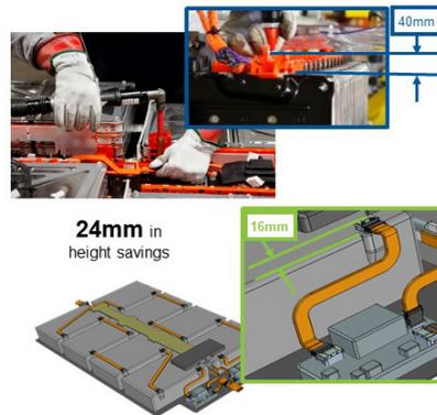
**The push/click/plug mate solution nature of the RigiFlex connection system allows the copper contacts at the end of the busbar to be completely enclosed. This promotes safety by eliminating risks for inadvertent shock.**
